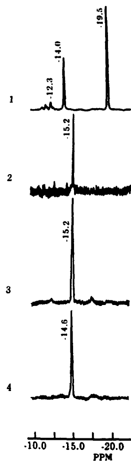
Fig. 2. ^{31}\text{P} NMR spectra of CePW at room temperature: (1) – 5 wt% aqueous solution, pH 2.5–3.0, (2) – saturated solution in n-BuOH ( 0.15 \text{ g l}^{-1} ), (3) – MAS spectrum for solid CePW pre-treated at 250^\circ\text{C} for 2 h, (4) – MAS spectrum for solid CePW recovered after reaction (dried in vacuo at 50^\circ\text{C} ).
